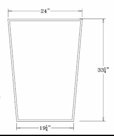
Top Diameter is 24". Middle diameter is 21". Bottom diameter is  $19\frac{1}{4}$ "
