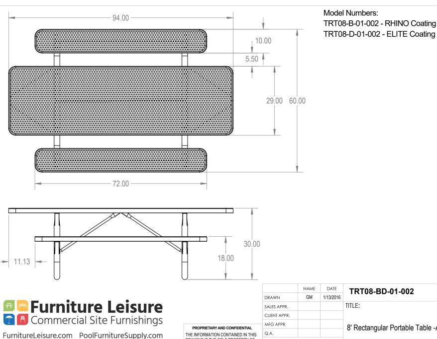
8' Rectangular Portable Table -Accessible Alt Q.A. THE INFORMATION CONTAINED IN THIS DRAWING IS THE SOLE PROPERTY OF Design By -Aadvantage Panels & Fence, Inc. PO Box CADWorksPro 1790 Whitney, TX. ANY REPRODUCTION **Punched Steel** IN PART OR AS A WHOLE WITHOUT THE Chicago, IL WRITTEN PERMISSION OF Aadvantage Panels & Fence, Inc. PO Box 1790 Whitney, www.cadworkspro.com WEIGHT: SHEET 3 OF 3 3 2
