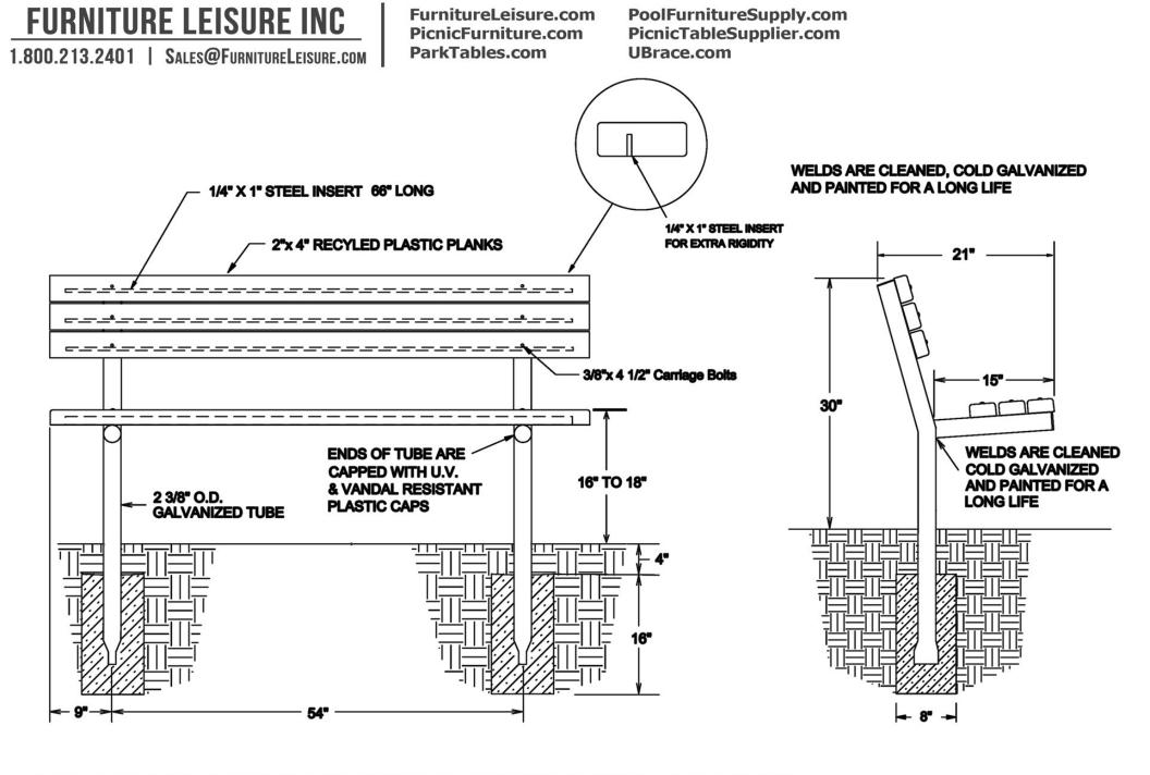
NOTE: THE BURY DEPTH OF THE CONCRETE FOOTING IS ONLY A SUGGESTION THE LOCAL SOIL CONDITIONS SHOULD DETERMINE WHAT IS NECESSARY
