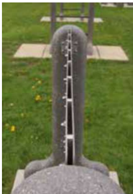
Sideview showing stainless steel divider bars.
