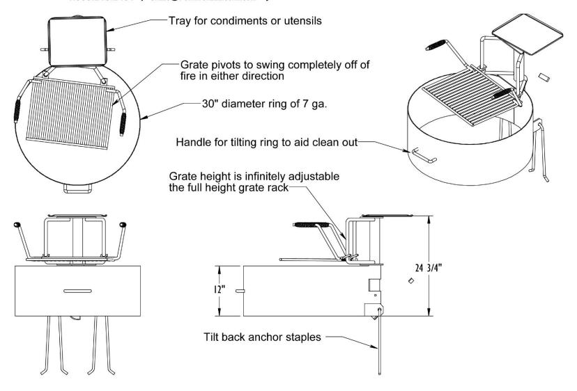
The fully adjustable grate allows for the *ultimate* grilling and cooking experience. The grate height is infinitely adjustable.
