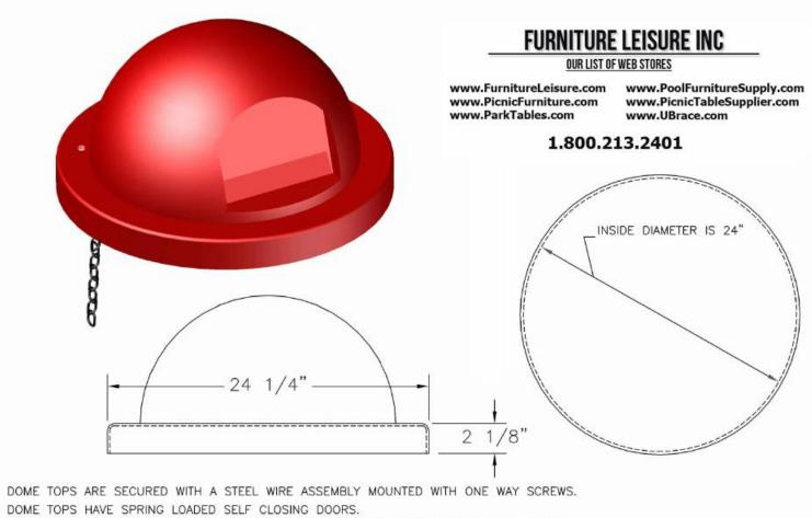
DOME TOPS HAVE SPRING LOADED SELF CLOSING DOORS.
