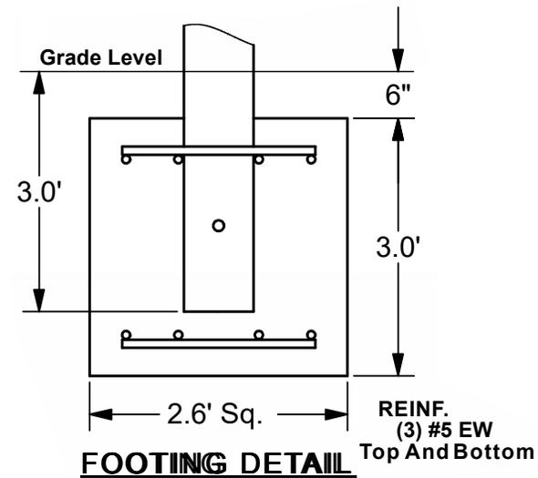
\*Footing design based on 1500 PSF soil bearing pressure.
