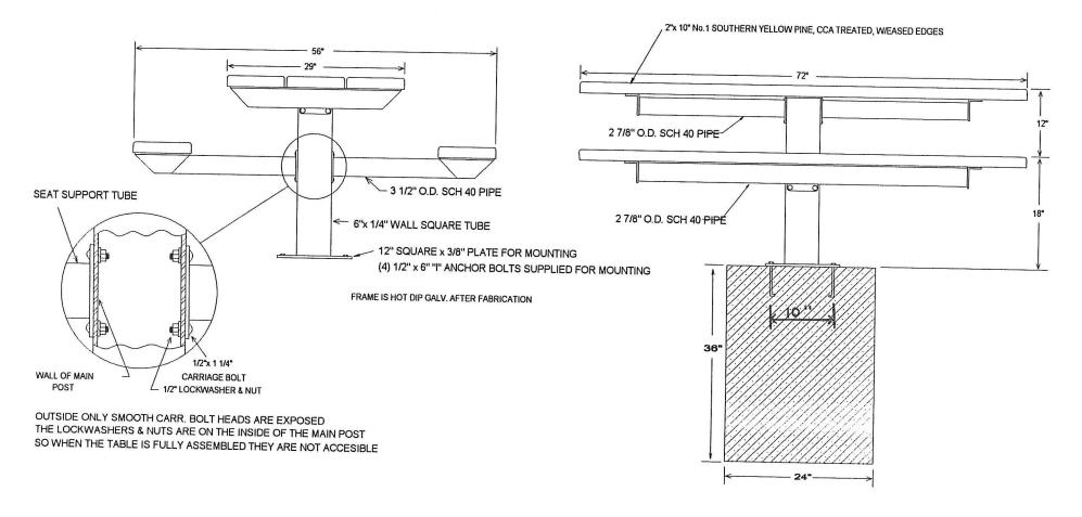
THE SIZE OF THE CONCRETE BASE IS ONLY A SUGGESTION YOUR LOCAL SOIL CONDITIONS SHOULD DETERMINE WHAT IS NECESSARY TO ENSURE A STABLE MOUNTING
