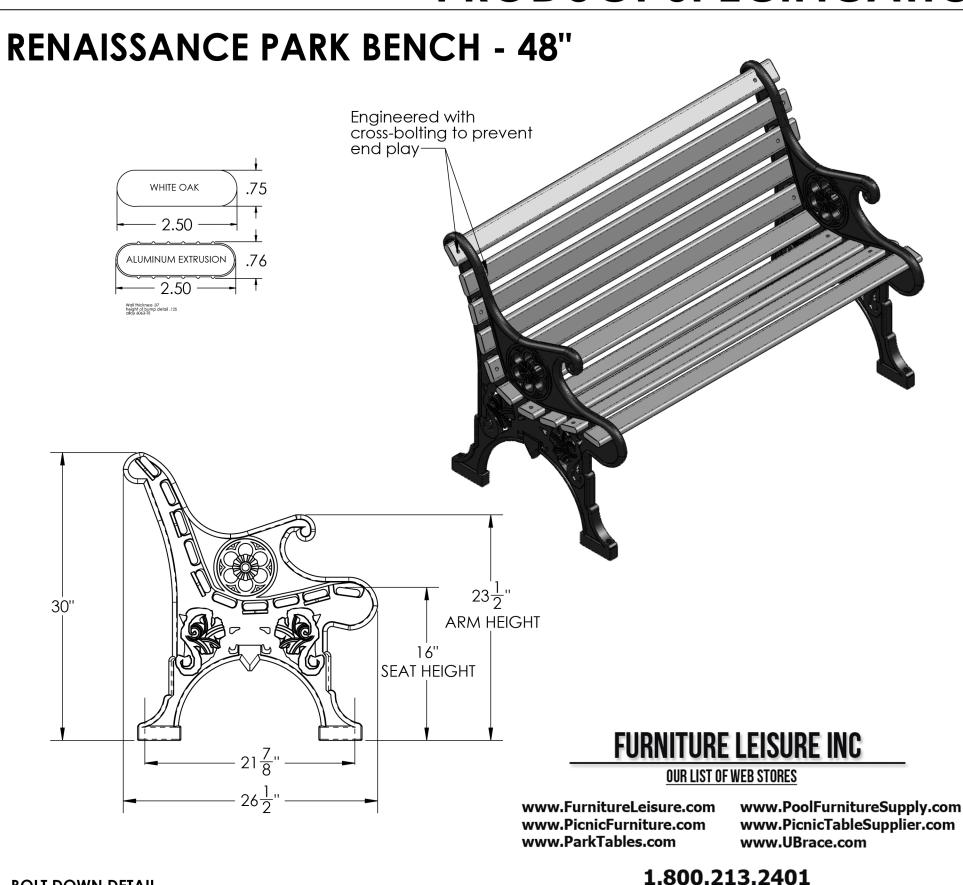
Material: Cast aluminum poured in permanent molds Finish: Electro static powder coating Color: Black, White, Green, Tan, Dk. Brown, Dk. Green, Bronze and Blue.
