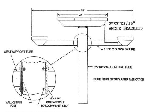
OUTSIDE ONLY SMOOTH CARR. BOLT HEADS ARE EXPOSED THE LOCKWASHERS & NUTS ARE ON THE INSIDE OF THE MAIN POST SO WHEN THE TABLE IS FULLY ASSEMBLED THEY ARE NOT ACCESIBLE
